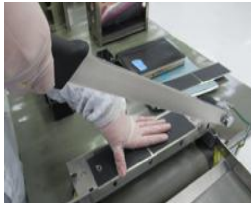
Fig. 3. Thumb was wrongly placed at cutting area of the jig
