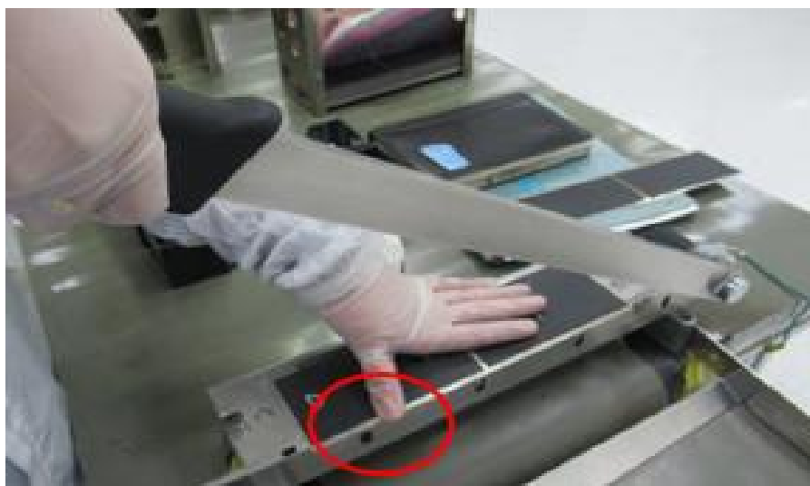
Fig.10 Safety risk Involved for manual derail
