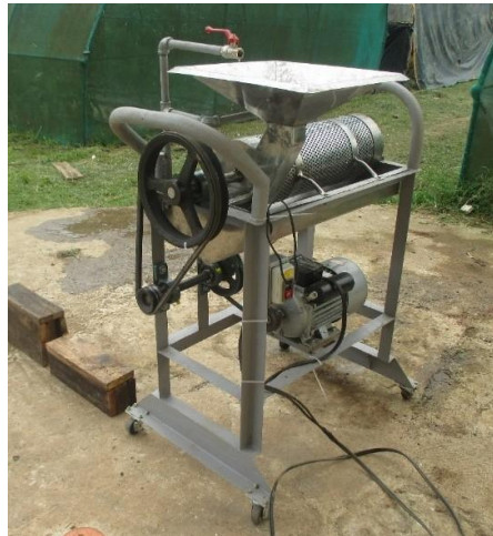
Fig. 3. Fabricated demucilaging machine
